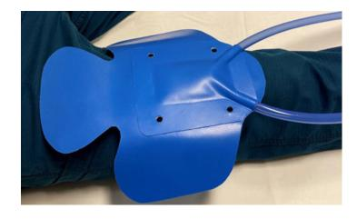
Position the Pillow Passive Driver and secure firmly with the adjustable belt assembly.
