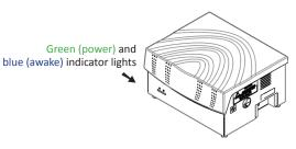
NOTE - INDICATOR LEDs: The Active Driver front panel includes a green indicator light for Power and blue indicator light to indicate Awake (ready to output acoustic energy). Both lights should be illuminated prior to and during an MRE exam. If the Awake light is not illuminated, turn the Active Driver off for five (5) seconds and then back on, or input a UDP command over the Ethernet channel in order to reset the Active Driver to an Awake state.
